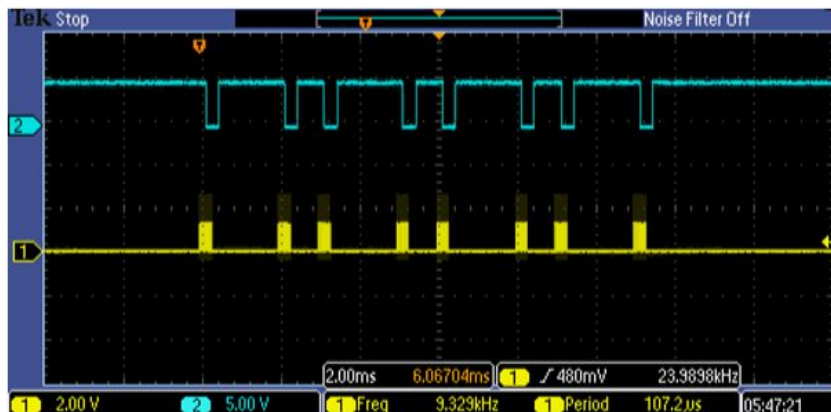
Figure J2. Output from MCU and TSOP18456
