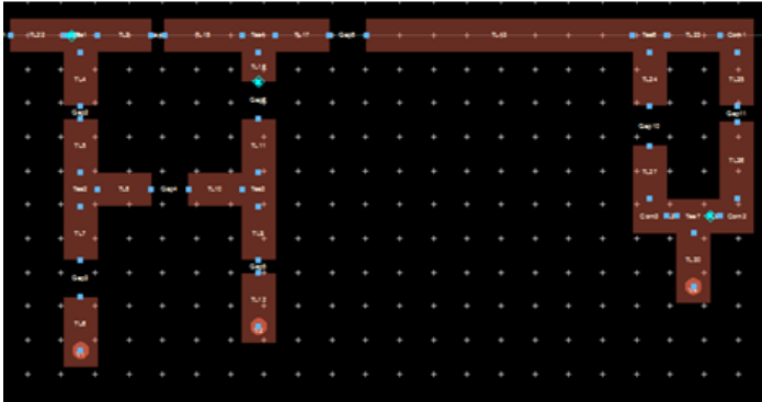
Fig. 3.9. Layout of 2-Stage charge-pump with on-board load (not to scale)
