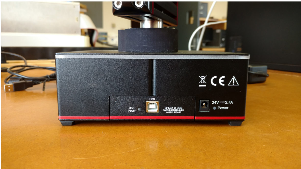
Figure C.1: QFLEX 2 USB panel installed on the Quanser AERO.
