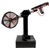
Figure: Quanser AERO configured as 2-DOF helicopter. Image courtesy of Quanser [8].
