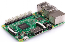
Figure: Raspberry Pi 3. Image courtesy of the Raspberry Pi Foundation [2].
