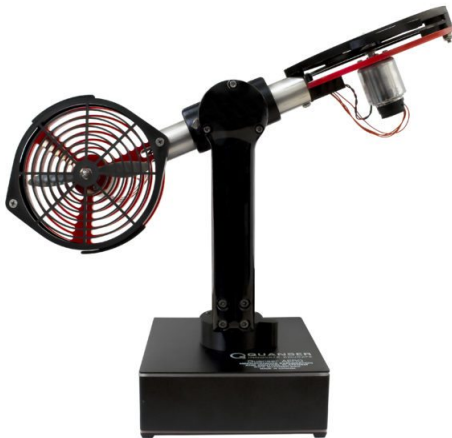
Figure: Quanser AERO configured as a 2-DOF helicopter.
