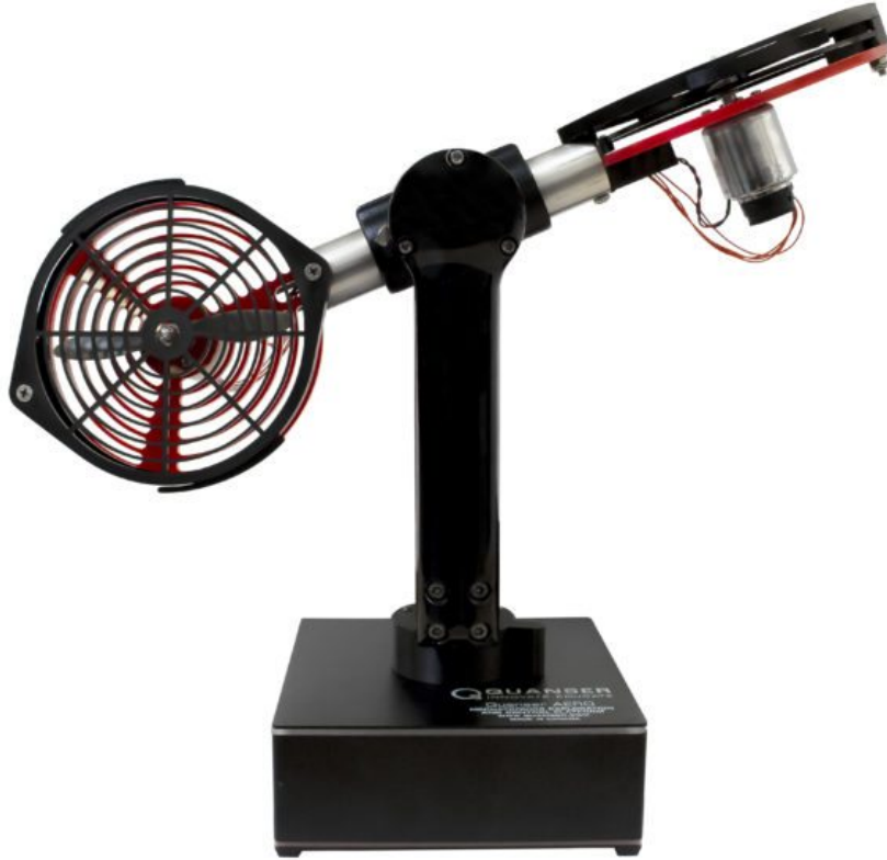
Figure 1: Quanser AERO configured as 2-DOF helicopter.
