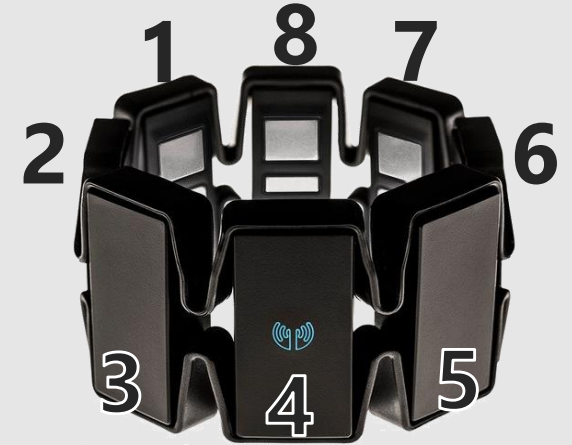
Myo Gesture Control Armband with labeled sensors
