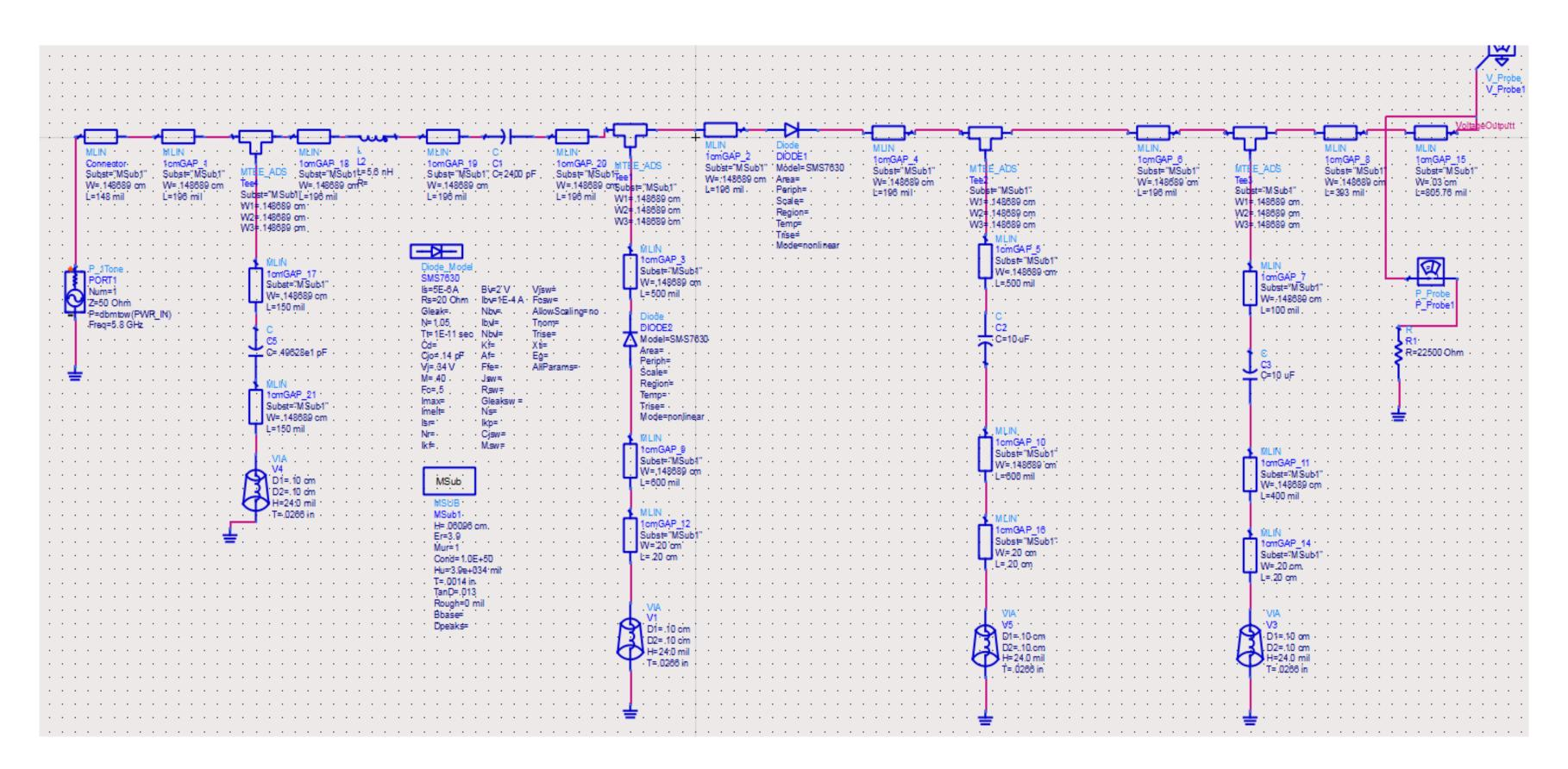
The original generic design generated great results for the system output. Once the microstrips were added the simulations drastically changed from outputs of 1.4V to outputs of .05V. After boosting inputs and adjusting microstrip lengths, the voltage did boost back up to the required voltage but ripple of voltage was nearly .2V. Capacitor value changes and microstrip length adjustments on the breakout strips generated an output voltage of 1.2V with only .08V of ripple.
