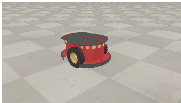
Figure 3.1: Pioneer 3-DX model used in V-REP simulations.
