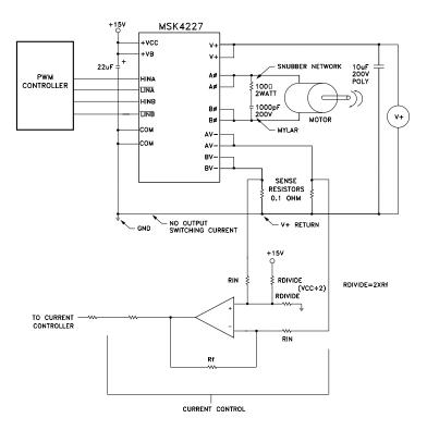
This is a diagram of a typical application of the MSK4227. The design +Vcc voltage is +15 volts and should have a good low ESR bypass capacitor such as a tantalum electrolytic. The digital inputs can come from a microprocessor or any type of PWM controller. The controller will use the current sense signal to either control current through PWM, current limit the bridge, or both.
