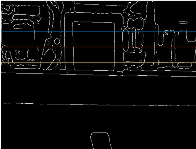
The team member tried to solve this problem by blurring the image prior to edge detection and using the Sobel method instead of Canny. These two changes result in much less background noise, but also less detail in the foreground. The resulting image is shown below. It may be useable, but a new method of measurement is needed.
