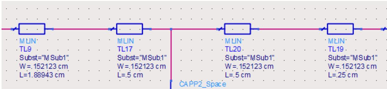
Fig. 9 ADS Design of Output Microstrip Spacing
