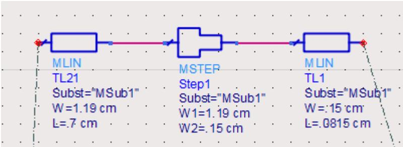
Fig. 5 ADS Schematic Design for Impedance Matching Network
