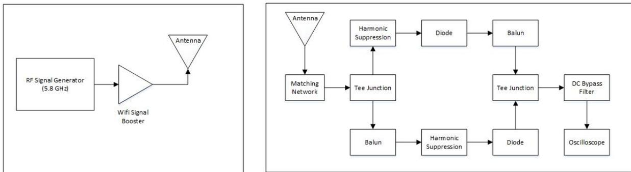
Fig. 4 Block Diagram of Wireless Power Transfer System. Transmitting Block on left and Receiving Block with RF to DC Converter on right
