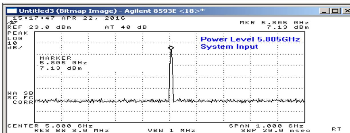
Fig. 20 Input Signal to RF to DC Converter
