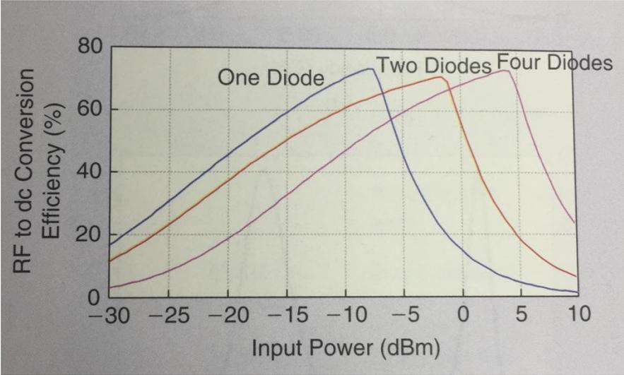
Fig. 1 Efficiency of Full Wave Rectifiers vs Input Power [1]
