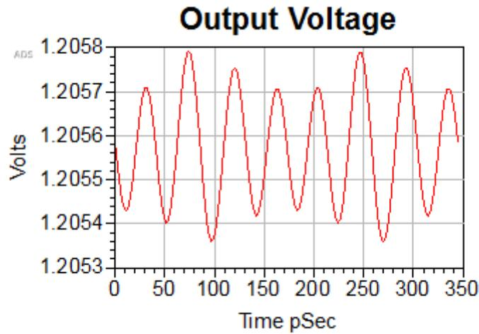
Fig. 14 Output Wave Form for ADS Schematic Simulation of unmatched converter
