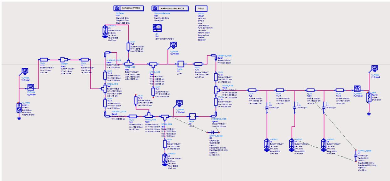
Fig. 15 ADS Schematic Design for Simulation of Matched Converter
