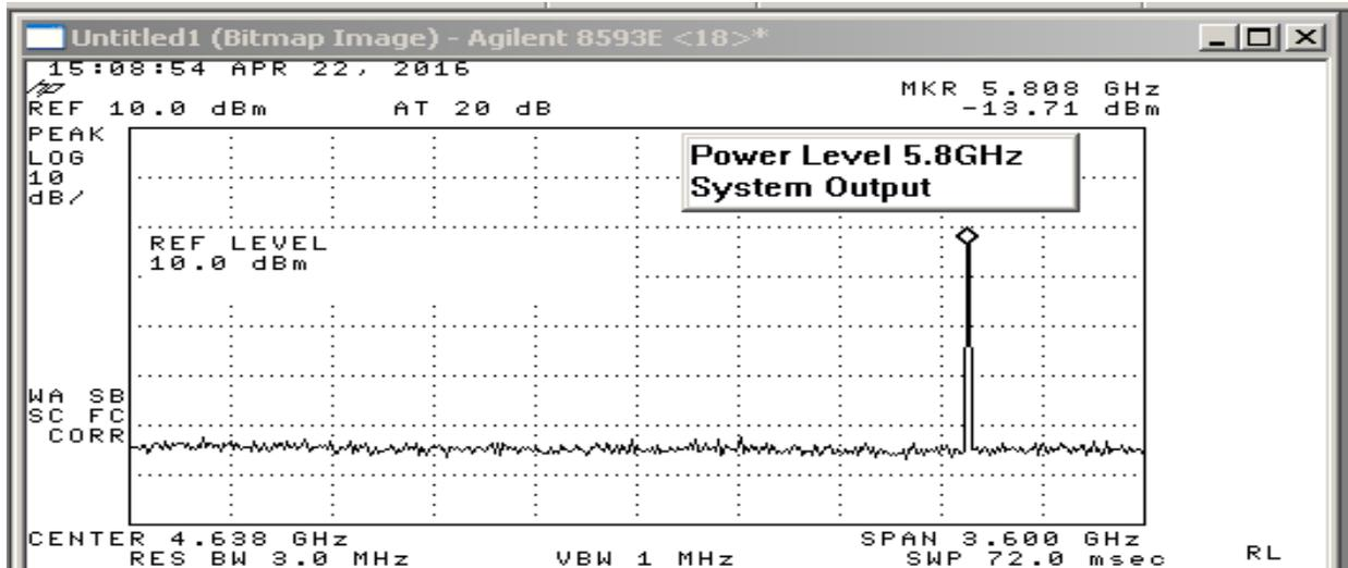
Fig. 21 Output Signal of RF to DC Converter
