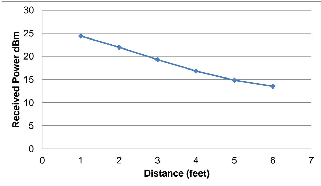
Fig. 22 Power Received at Varying Distances
