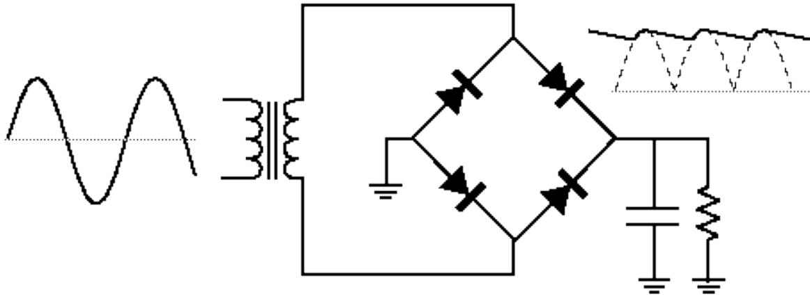
Fig. 2 Four Diode Full-Wave Bridge Rectifier
