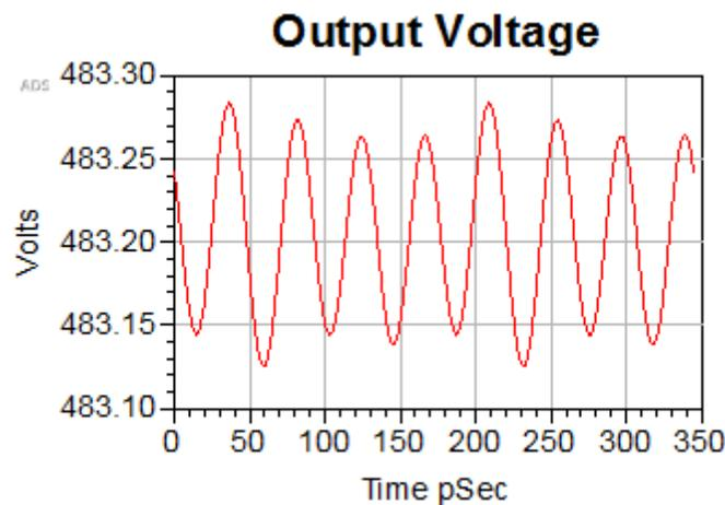
Fig. 18 Output Wave Form for ADS Schematic Simulation of Unmatched Converter (Voltage in mV)
