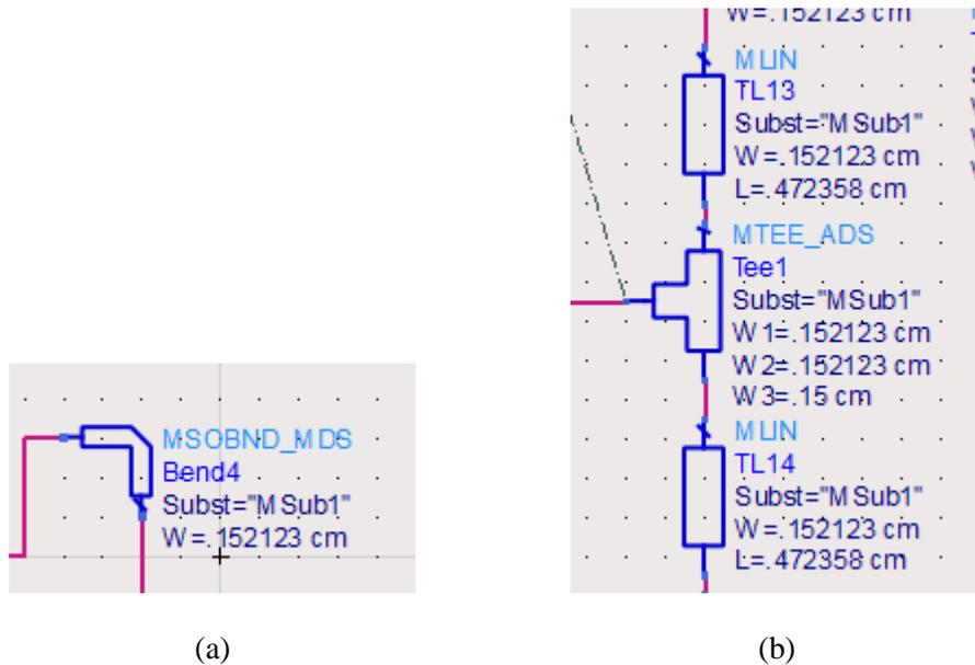
Fig. 10 ADS Schematic of Discontinuities Present in RF to DC Converter Project (a) Schematic Bend (b)
