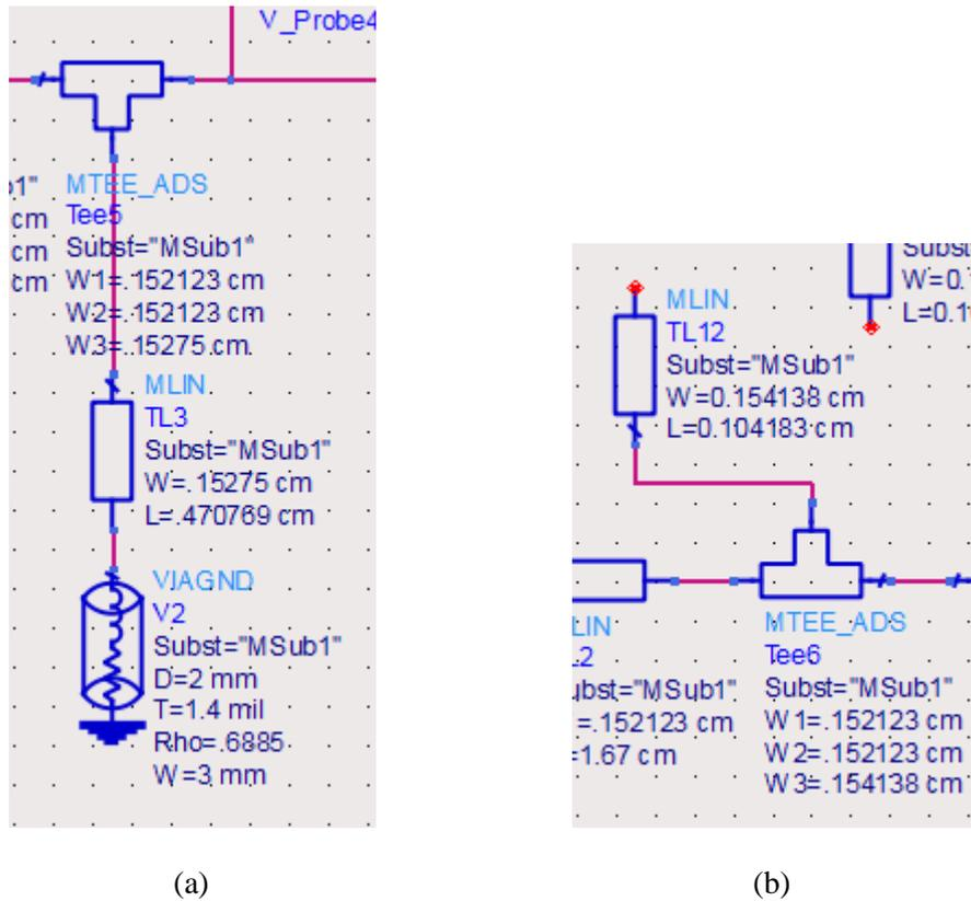
Fig. 7 (a) ADS Schematic of Second Order Harmonic Suppression; (b) ADS Schematic of Third Order Harmonic Suppression
