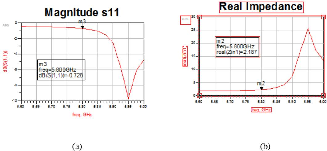
Fig. 12 ADS Simulation Results for Unmatched Converter. (a) Magnitude of Reflection Coefficient seen at input. (b) Real Impedance seen at input
