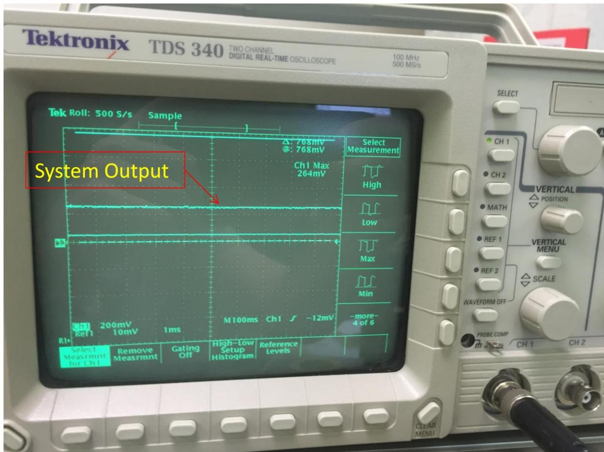
Fig. 19 Time Domain DC output of the RF to DC Converter Project
