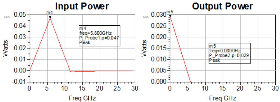
Fig. 13 Input Power vs. Output Power of unmatched converter ADS Schematic Simulations
