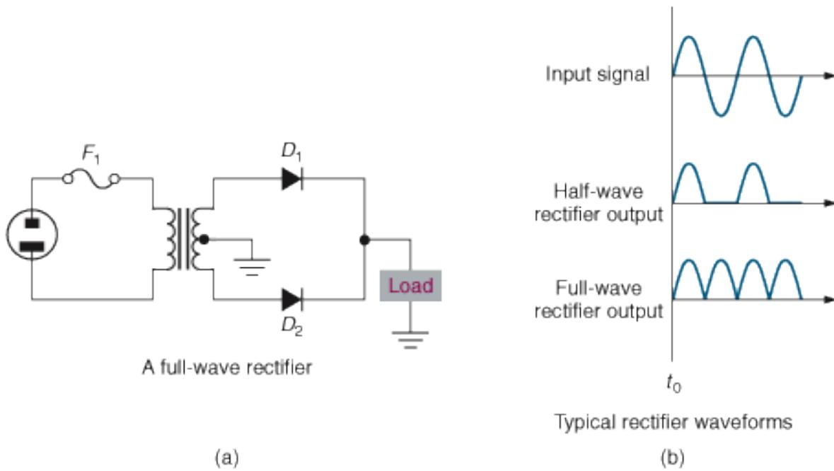
Fig. 3 Two Diode Full-Wave Rectifier
