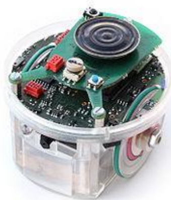
Fig. 7. Test Platform – E-puck [6]
