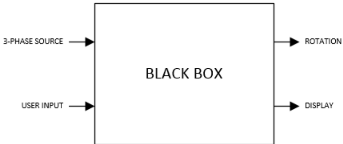
Fig. 1 System Block Diagram showing the necessary inputs and outputs of the system
