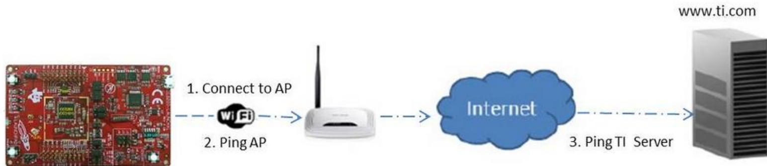
Figure 23. CC3200 set up in station mode [10]
