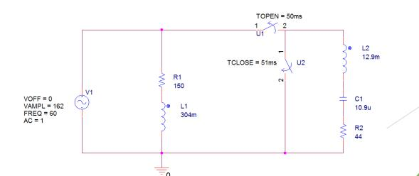
Final design for the tuned 7<sup>th</sup> harmonic filter using a RLC circuit
