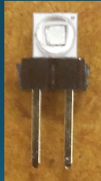
LED soldered to section of header pins
