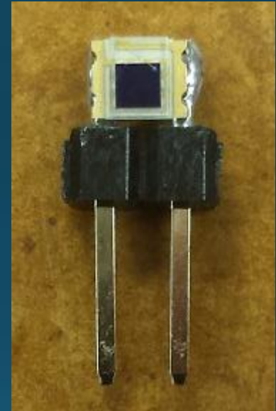
Everlight photodiode soldered to section of header pins
