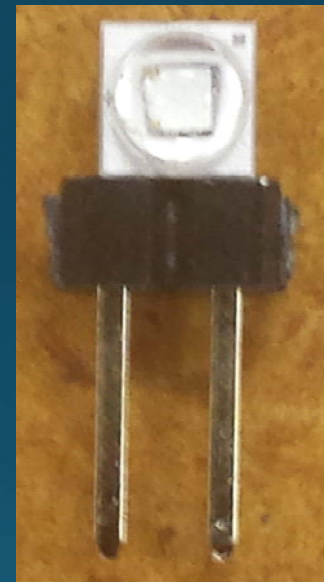
LED soldered to section of header pins
