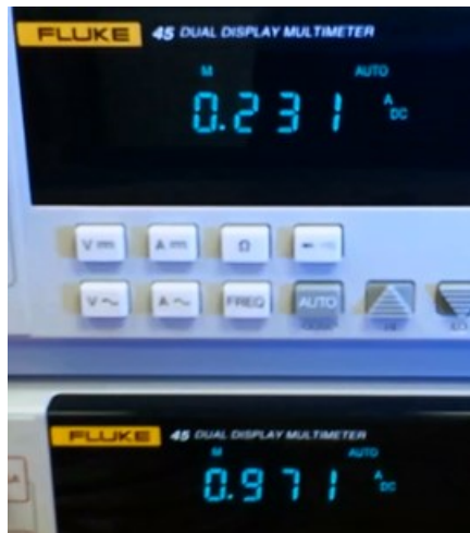
Fig. 28. The bench-top average current test readings. The 3 cell NIMH supply is on top.
