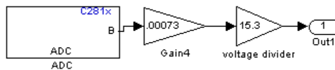
Figure 16: The ADC and voltage divider multiplier block
