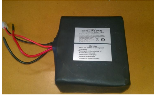
Figure 11: 51.8V Li-Ion Battery (Large Scale Testing Battery)
