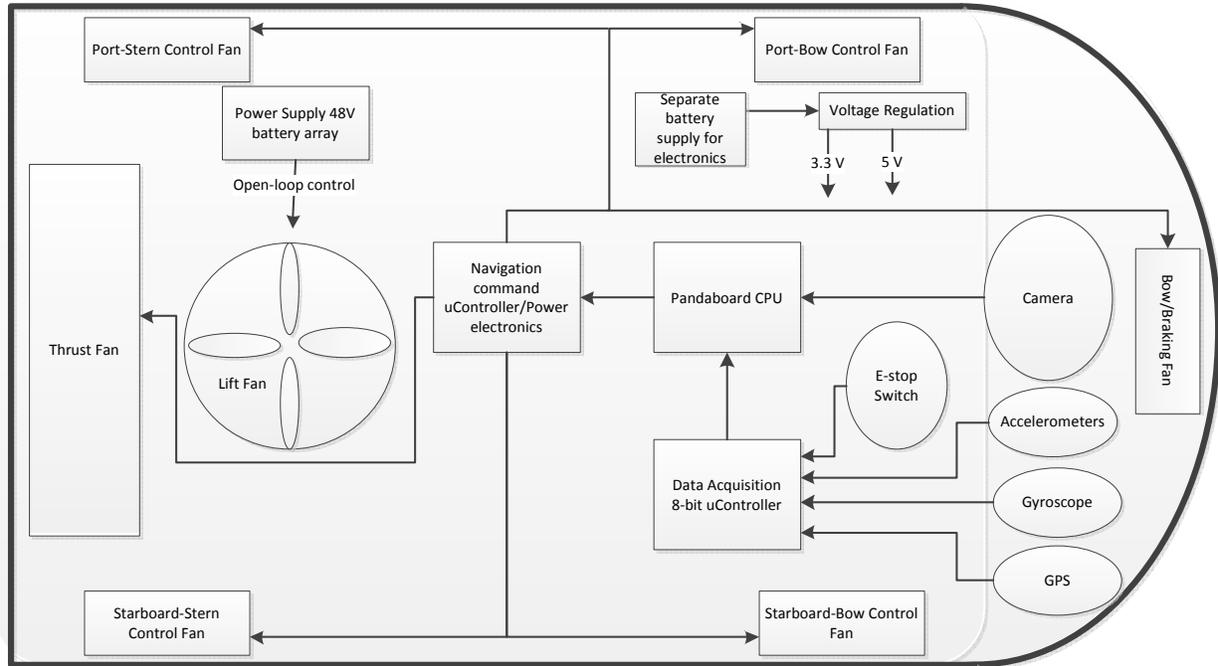
Figure 2-1 – Functional System Diagram for the NASTI
