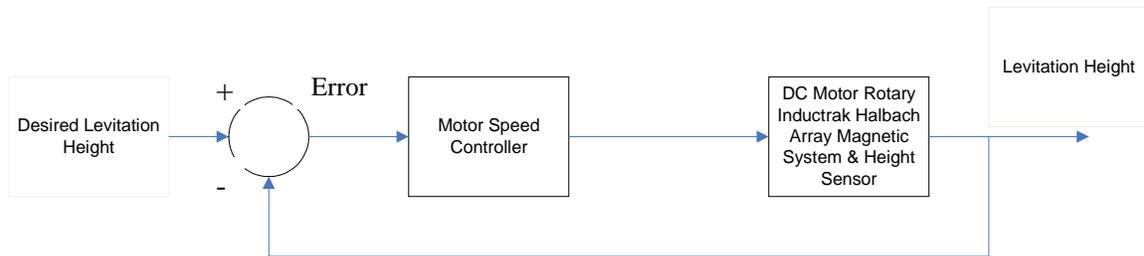
Figure 1: High level overall system block diagram
