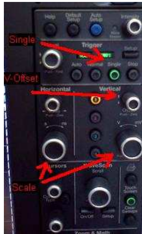
Fig. A14: Oscilloscope Buttons and Wheels
