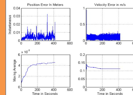
The unscented Kalman filter consistently finds an accurate estimate of the GPS solution for a single parameter set. The position is accurate up to within a few millimeters of the GPS and the velocity is accurate up to just over 10 centimeters of the GPS velocity.
