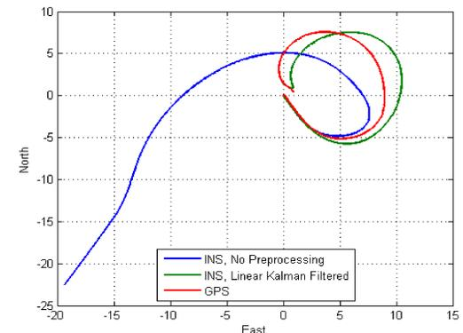
With much manual tuning, the linear Kalman filter can find a more accurate solution than the standard INS, but the nonlinearity of the system
