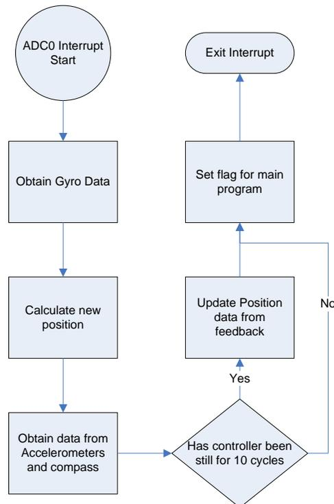
**Figure 9: A/D Interrupt Flowchart**
