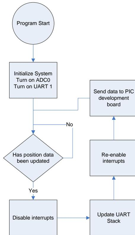
**Figure 8: Main Loop Flowchart**
