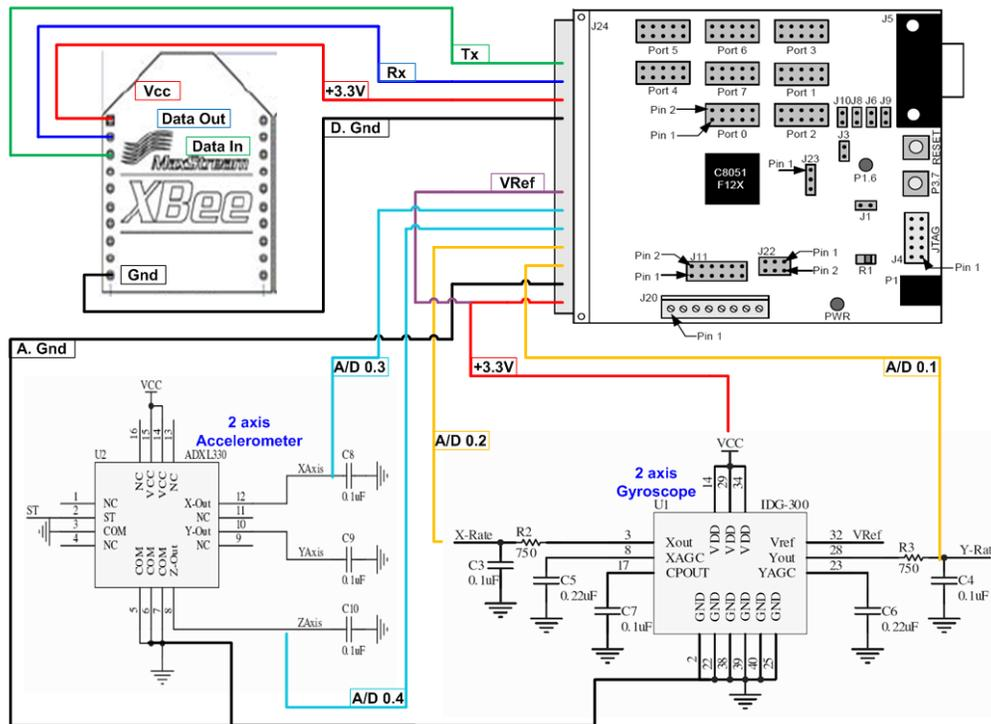
Figure B-1: Inertial Board Schematic
