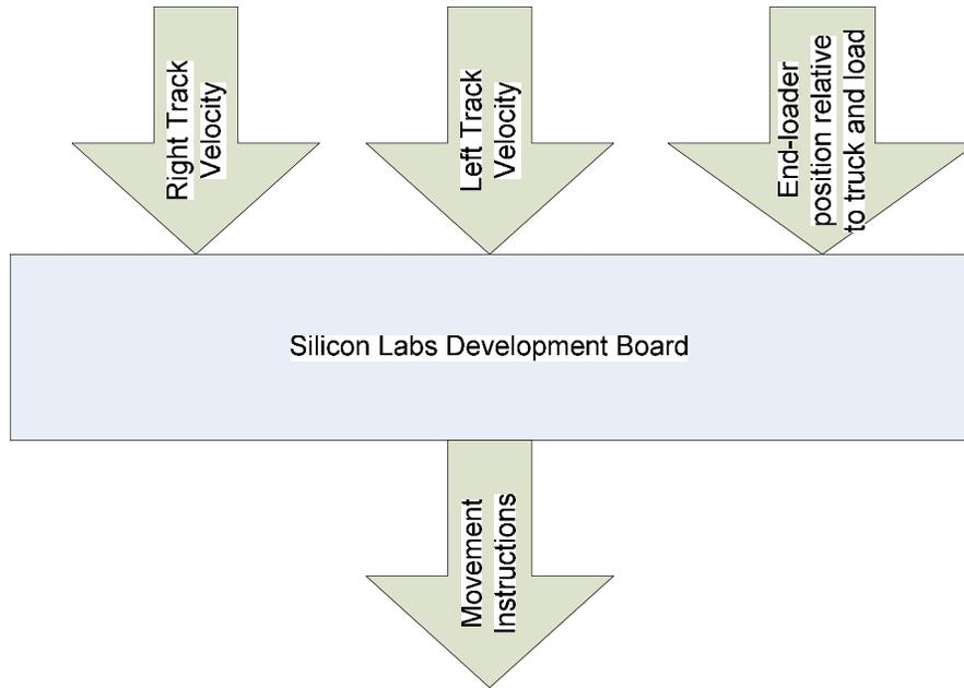
Figure 4: Development Board Subsystem Block Diagram
