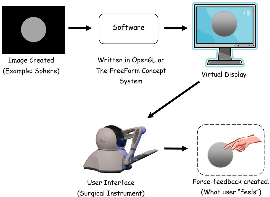
Figure 2-1: High Level Overall System Block Diagram
