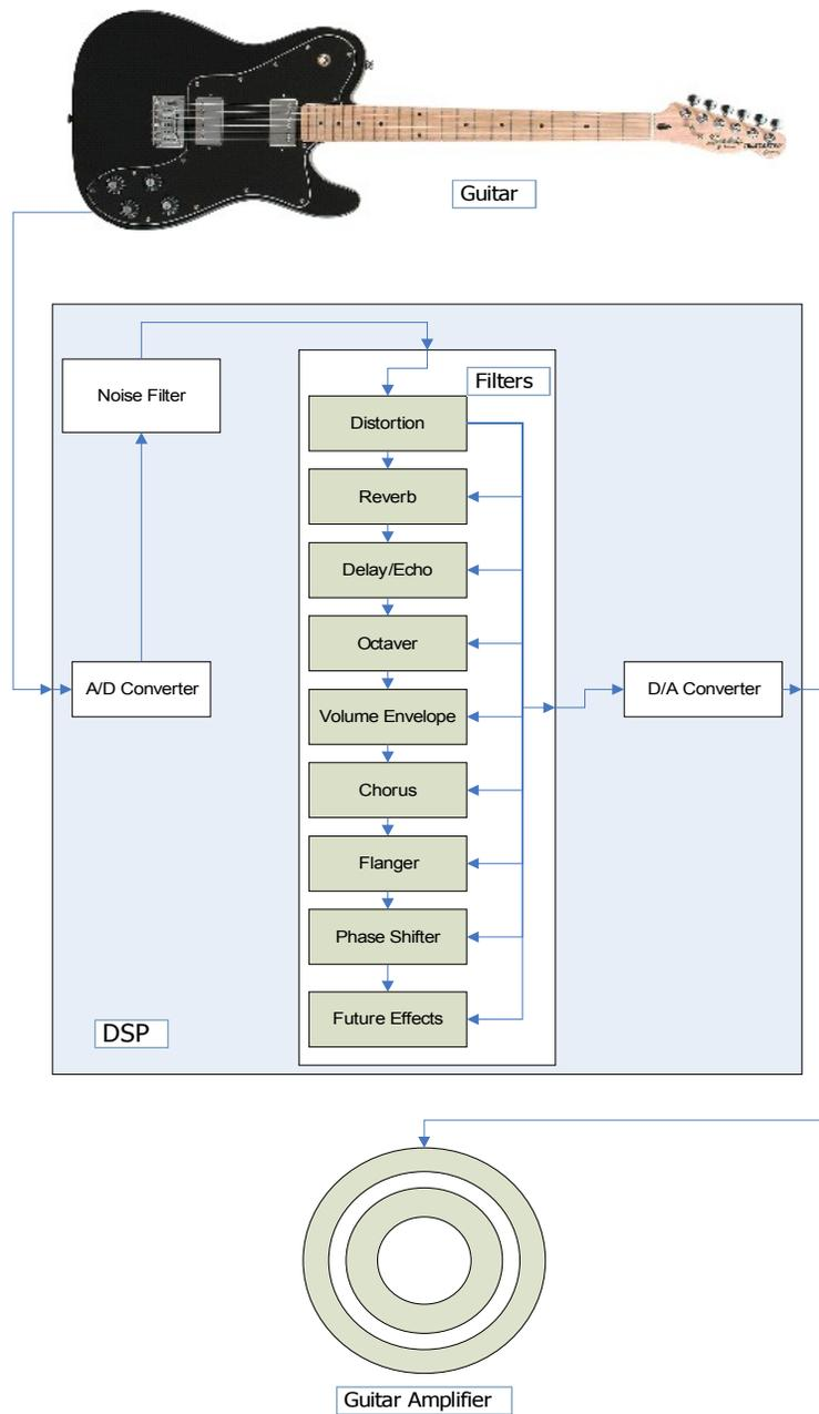
The signal comes from the guitar and goes to the DSP. It is converted to a digital signal first, then it passes through a noise filter. From the noise filter, it goes to the user-defined effects filters. After this, the modified signal is converted back to analog and is sent to the guitar amplifier for sound generation.
