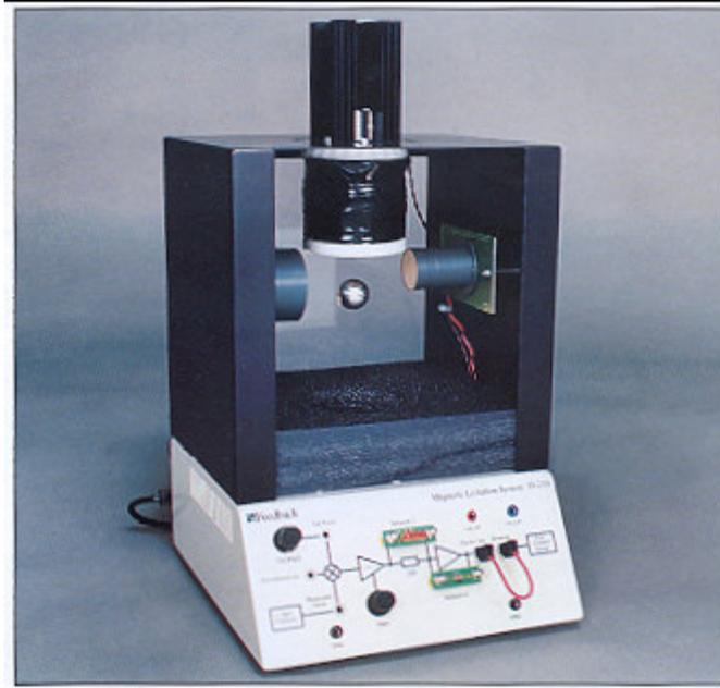
Figure 2: Photo of Magnetic Suspension Plant
