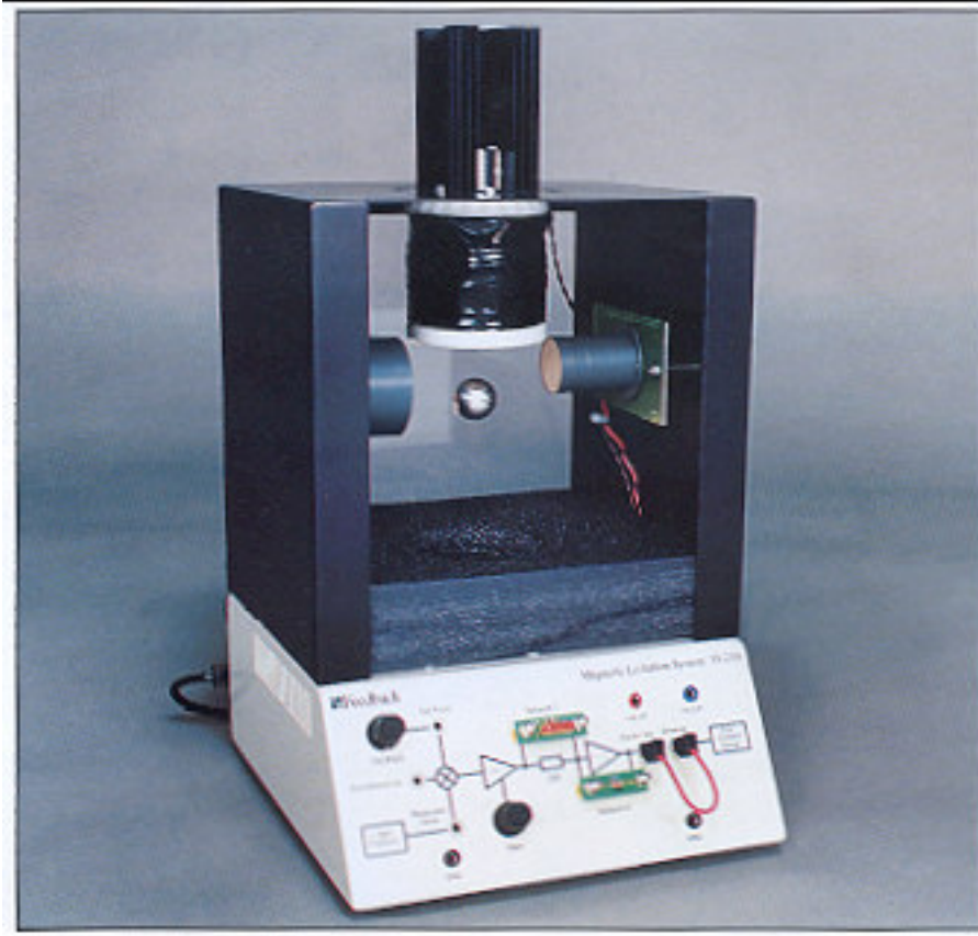
Figure 5-1: A photograph of the Magnetic Suspension System
