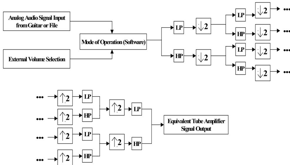
**Figure 4: Multirate Signal Processing Approach to Tube Amplifier DSP Model**
