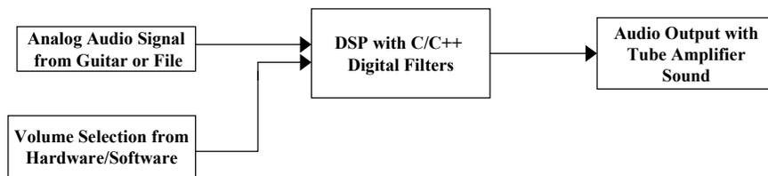
**Figure 1: Overall Block Diagram**
