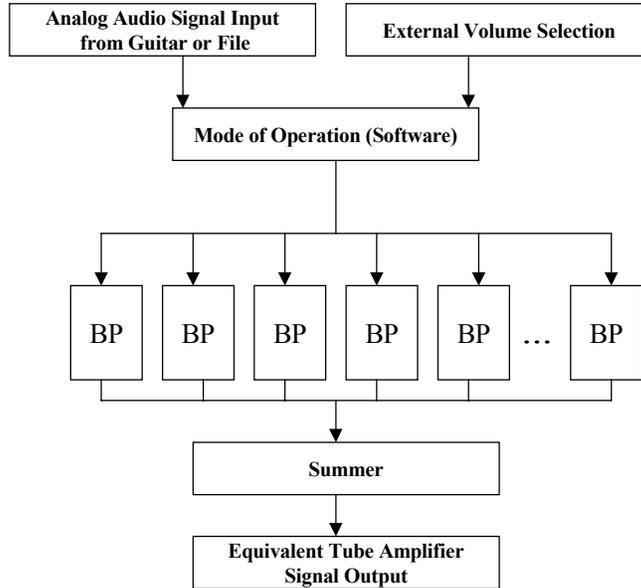
**Figure 2: Multiple Bandpass (BP) Digital Filter Approach to Tube Amplifier DSP Model**
