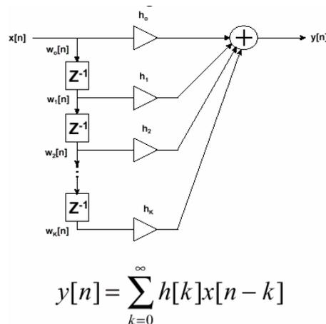
**Figure 5: FIR Digital Filter Algorithm**
