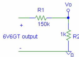
$$V_o = (R_2 / (R_1 + R_2)) * 6V6GT \text{ output} = 0.00662 * 6V6GT \text{ output}$$
