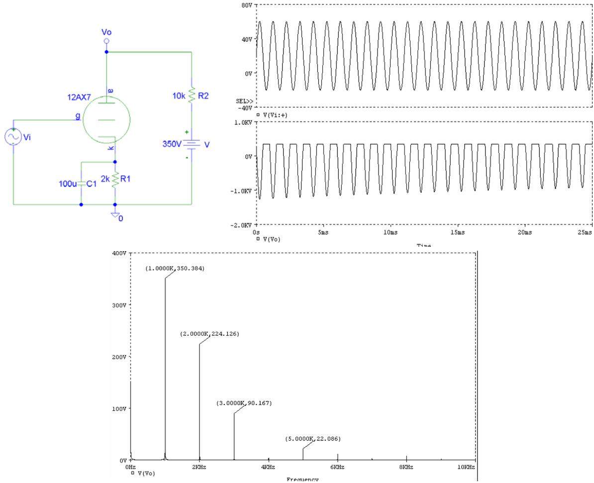
Figure 7: 12AX7 Triode PSPICE Transient Analysis Simulation Results
