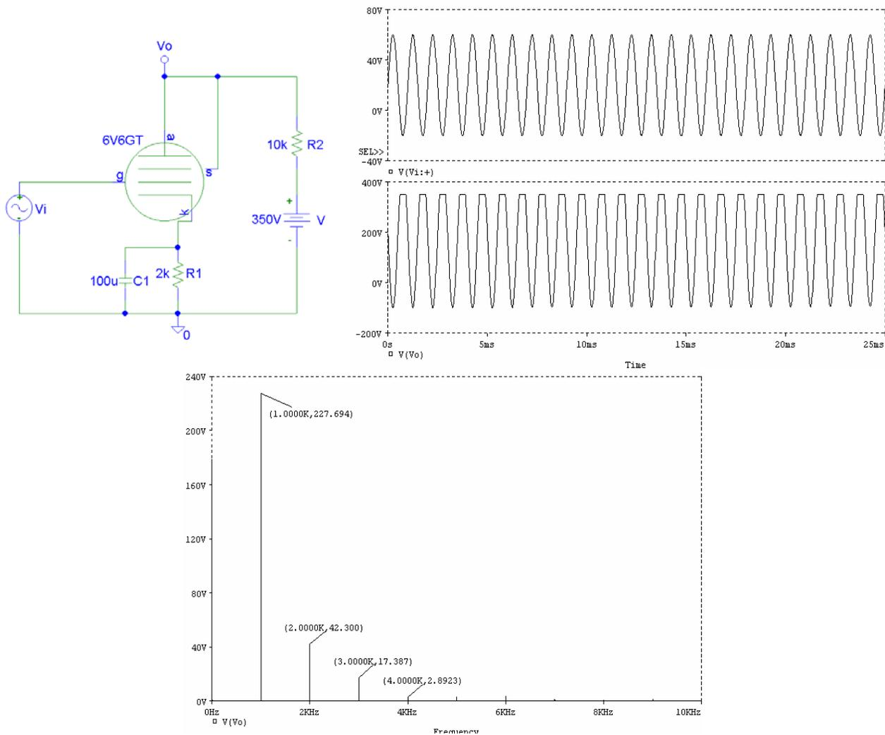
**Figure 8: 6V6GT Pentode PSPICE Transient Analysis Simulation Results**
