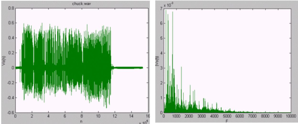
**Figure 12: Fender Champ Output from a 1952 Telecaster Input**
