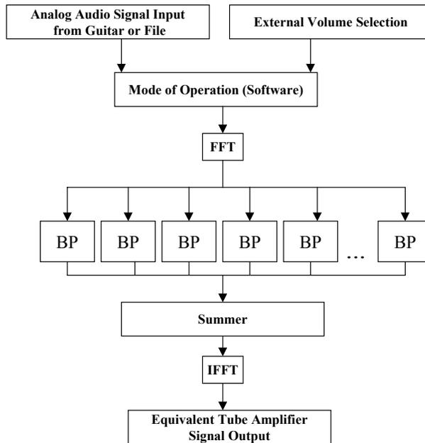
**Figure 3: FFT Filter Network Approach to Implement a Bandpass (BP) Filter Bank for Tube Amplifier DSP Model**
