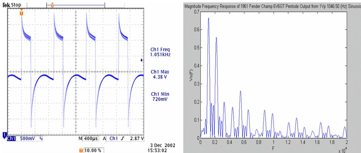
**Figure 11: Output at Single-Ended Power Tube Stage of 1961 Fender Champ at Volume 12 for a 1Vp, 1046.50 (Hz) Sinusoidal Input**
