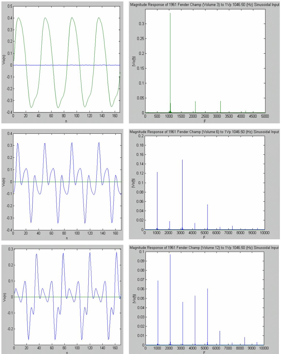
**Figure 9: Fender Champ Output in 16-bit Digital Audio Data for 1Vp 1046.50 (Hz) Sinusoid at Volumes 3, 6, and 9**
